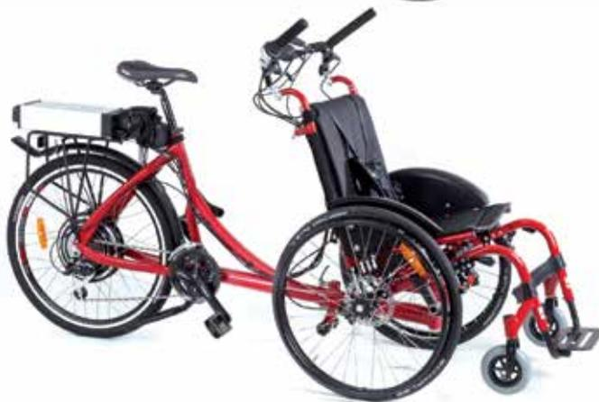
**Wheelchair tandems** (*below left*) have a heavy-duty wheelchair as the main component of the machine, onto which is attached a propulsion unit which resembles the back end of a regular bike. They are most suitable where only one person is to ride as passenger, such as a family with a disabled person. These are lighter and smaller than wheelchair transporters - and usually come apart for easy transportation..
